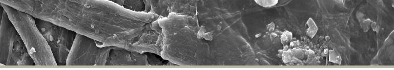
The abrasive effect of calcium carbonate on the headbox (wiring), felts and other machine parts of the paper machine depends upon the morphological stiffness and grain size of its particles. PCC has the advantage of greater volume and higher stiffness; the reason why many papermakers prefer to use PCC as a filler. On the other hand, GCC is preferred for coating because it possesses far better rheological properties. However, both products are equally suitable for either application methods.
